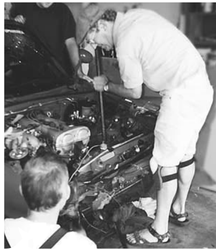
Richard looks on as a dapper Ken Evory uses a pry bar in preparation to removing his Sebring Supercharger.
