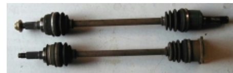
The halfshaft for the Torsen differential (top) is readily distinguished from the non-Torsen unit. The splined shaft fits into gears inside the Torsen unit.
