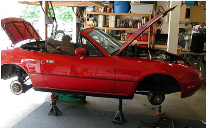
Left— The Miata of the Tech Day host, Wes Tewksbury, stands ready to receive all new adjustable shocks.
