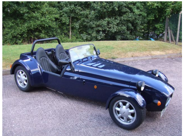
Westfield's latest kit car utilizes several Miata components. Notice the early NA wheels. Photo: Westfield Sportscars Ltd.
